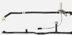
6 Battery Thermal Plastic Lines and Connectors
